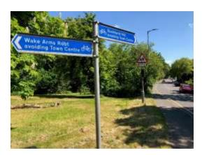
Sign post not straight, and the blades have been moved, so pointing in incorrect direction. I would suggest that the sign post be relocated to the rear of the litter bin, to protect from high-sided traffic turning the corner.
